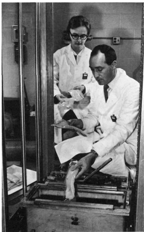
The fillets are placed in the ^{60}\text{Co} research irradiator at MIT to prolong their shelf life by radiopasteurization.
